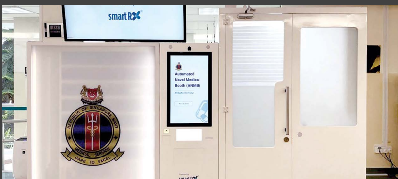
The Automated Naval Medical Booth (ANMB) capable of registration, triage and medication dispensary.
