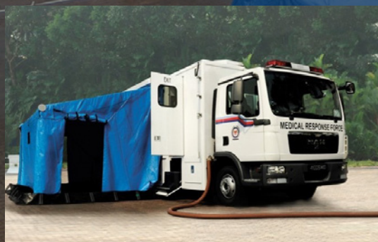
The Medical Decontamination and Treatment Vehicle: The decontamination configuration features two retractable side shelters with in-built roller tables and shower nozzles for casualties as well as one central compartment with an in-built shower system for multiple concurrent ambulatory casualties.
