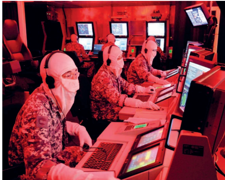
RSN ships are equipped with the locally developed Combat Management System. It is designed with embedded intelligence for track management, identification and weapon allocation functions, which improves decision-making in tactical war-fighting situations.
