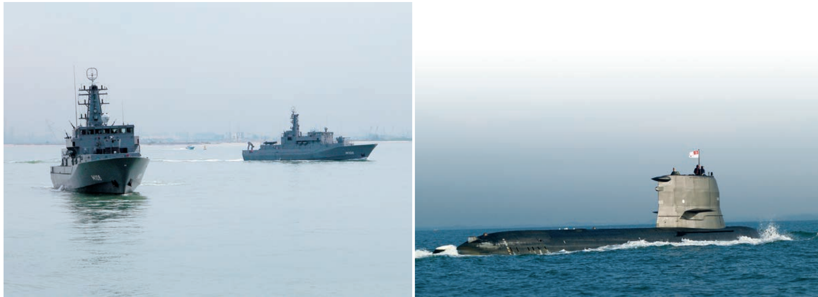
Left: The Bedok -class mine countermeasure vessels are equipped with mine disposal vehicles capable of detecting, locating, identifying and destroying modern sea mines. Right: The acquisition of the Challenger -class submarine in 1996 gave the RSN a newfound ability to operate in the underwater dimension.
