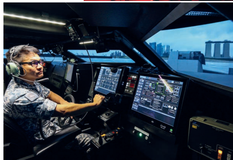
Below: ME3 To Yan Chern, deputy boat commander of a specialised marine craft, conducting navigation training at a simulator, which mimics the craft's cockpit. Here, the crew is able to train as a team to navigate and respond to emergencies.
