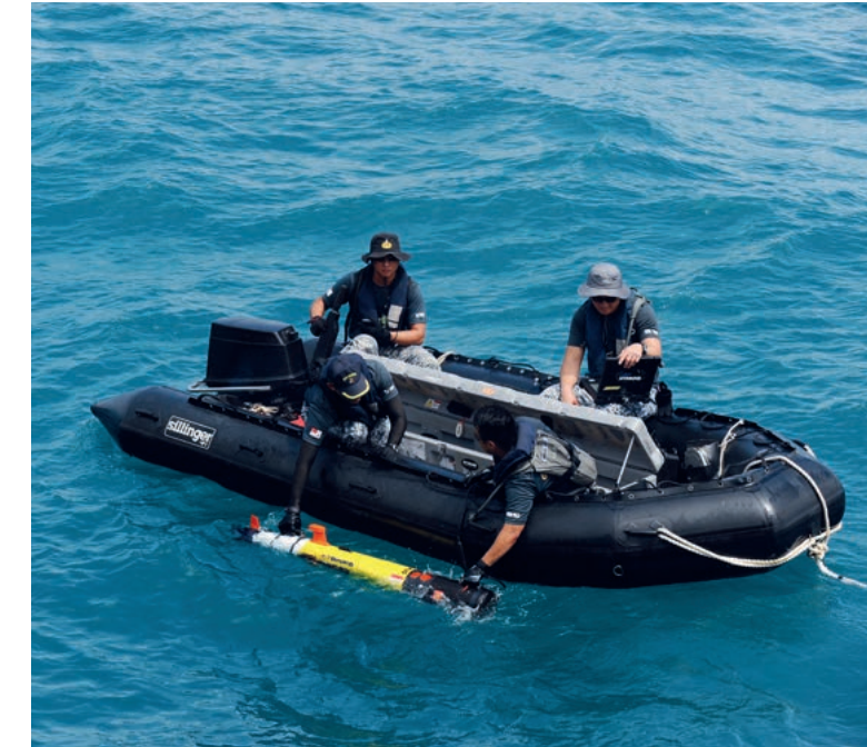
Since 2011, the REMUS Autonomous Underwater Vehicle has been deployed for exercises and operations, such as the search for AirAsia flight QZ 8501.
